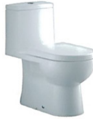
Aquarius Washdown One Piece Washdown WC1655 L 680 x W 355 x H 725mm 140mm (A) ; 225mm (S) 6/3 Litres, 4/3 Litres
