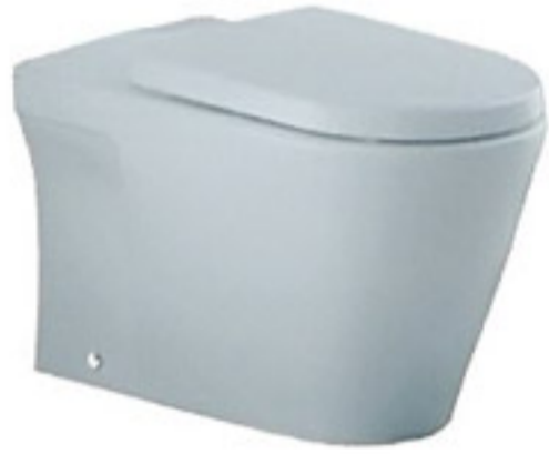
Venus Washdown Back To Wall Pan WC4709P L 620 x W 370 x H 390mm 6/3 Litres; S Trap Converter: 100mm Available in back / top inlet
