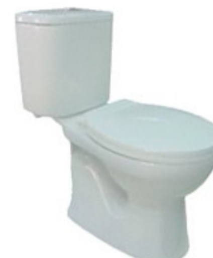
Iris Washdown Close Couple Pan WC4501 NS/P c/w LC3005ND BIBO L 700 x W 365 x H 800mm 260mm (S) ; 190mm (P) 6/3 Litres, 4.5/3 Litres
