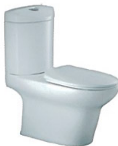
Leo Washdown Close Couple Pan WC4511S c/w LC3011DM L 700 x W 385 x H 800mm 260mm (S) ; 190mm (P) 6/3 Litres, 4.5/3 Litres
