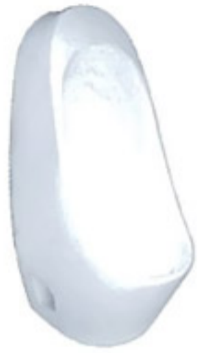
Long Boots Wall Hung Urinal UR5605 L 370 x W 325 x H 700mm Integral Trap with back / top inlet
