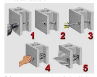
To fix anchors into hollow materials (bricks or blocks) perforated sleeves must be used.
